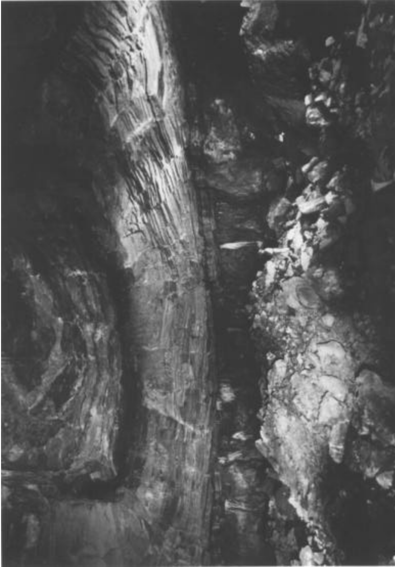
FIG. 26.4 Underground cavity created by the Gnome fusion explosion, part of the Plowshare program. Note the person standing near the center. (Courtesy of Lawrence Livermore National Laboratory, U.S. Department of Energy).
